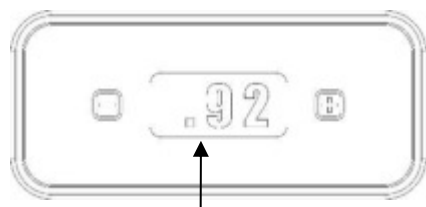
Temperature coffee boiler (t1, here 92°C) -period in the 1st position
